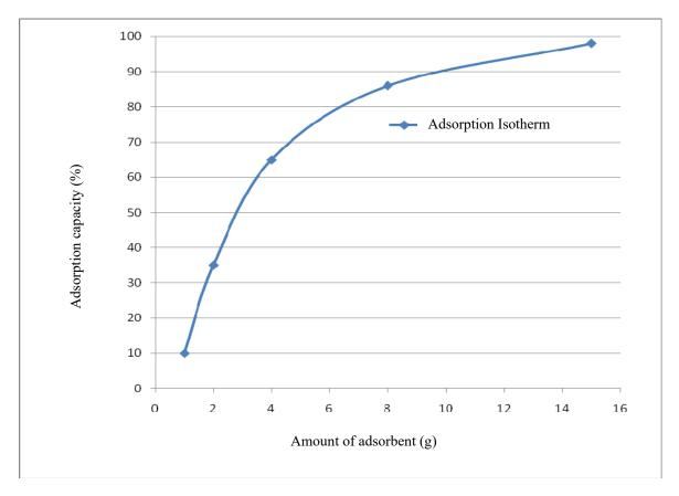
Figure 10. Typical adsorption isotherm of adsorbent (zeolite or bentonite) in terms of heavy-metal ions adsorption capacity (CAC, %) of adsorbent (zeolite or bentonite) as a function of adsorbent amounts (g)
