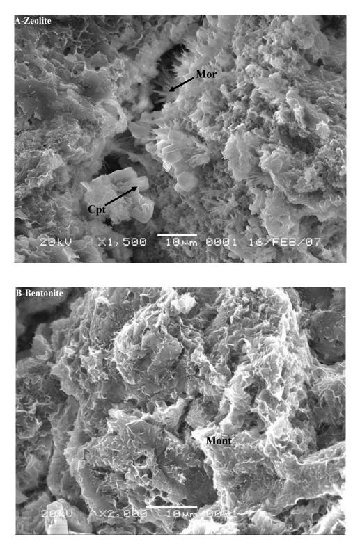
Figure 9. The SEM photomicrograph result of (A) the representative Gedangsari zeolitic tuff, showing the presence of zeolite minerals including clinoptilolite (Cpt) in tabular structure and mordenite (Mor) in fibrous structure (Idrus *et al.*, 2006; Idrus *et al.*, 2007), and (B) the representative Wonosegoro bentonitic tuff exhibiting the dominance of montmorillonite (Mnt) with its webby structure and other volcanic glasses (Titisari *et al.*, 2006; Titisari *et al.*, 2007)
